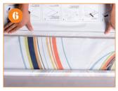
6. Arrange the graphic and the base leader parallel to each other, then peel off the adhesive paper.
